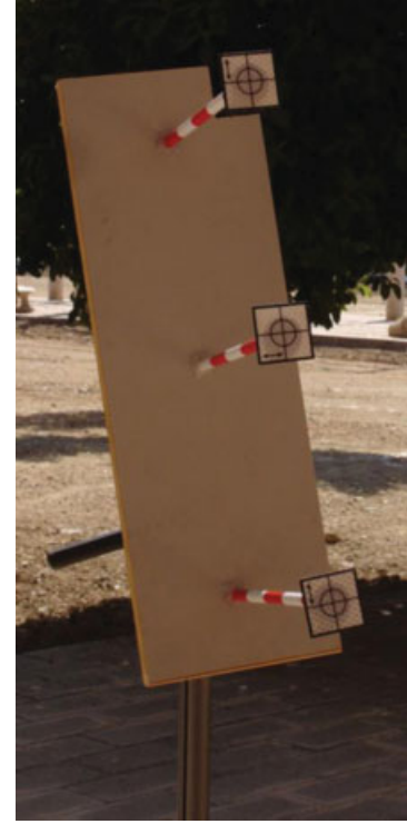
Fig. 8. Pattern for calibrating the laser scanner.
