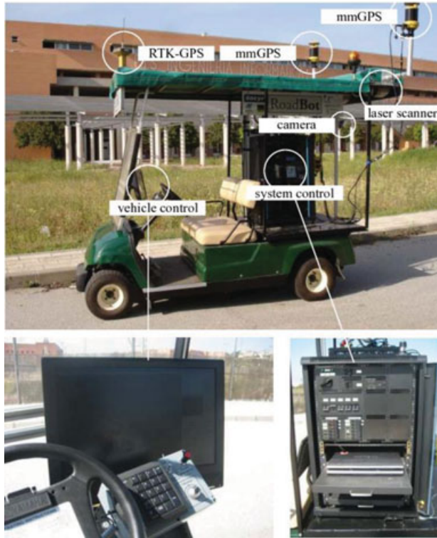
Fig. 1. The vehicle with the sensors and monitoring and control units.
